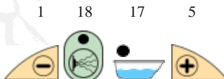
The whirlpool function can only be operated when the water level indicator is on.
