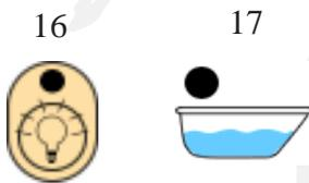
Key 16 turns the underwater light on & off. This can only be operated when the water level indicator is on.
