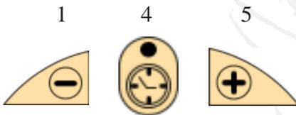
Press and hold key 4. After a few seconds the digital display will flash. Select the correct hour using keys 1 & 5. Press key 2 again and follow the same procedure to set the minutes. Press key 2 once more to save the time value and return to stand-by mode.
